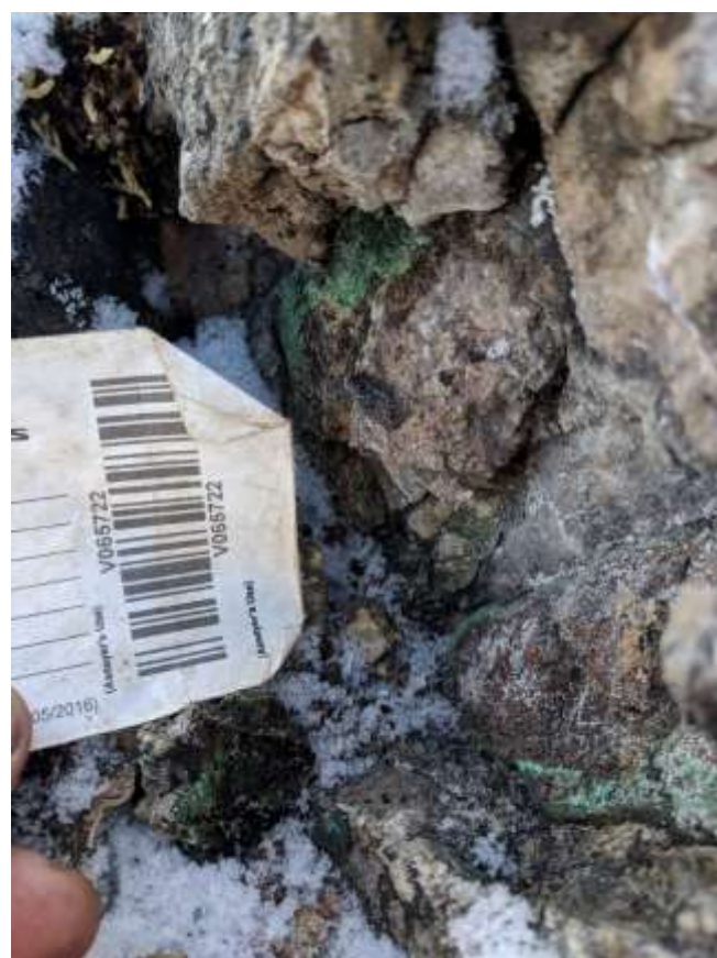
Blebs of chalcopyrite within calcite vein hosted by intermediate volcanic country rocks
