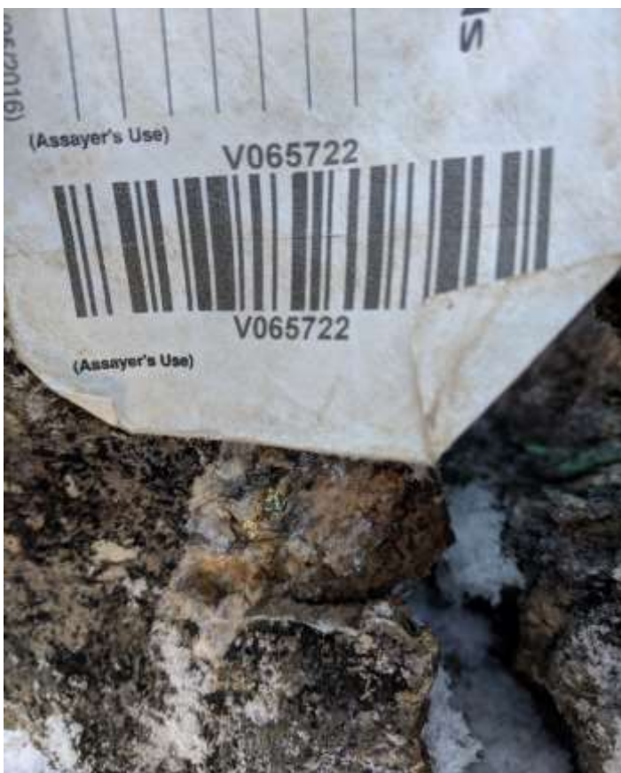
Blebs of chalcopyrite within calcite vein hosted by intermediate volcanic country rocks
