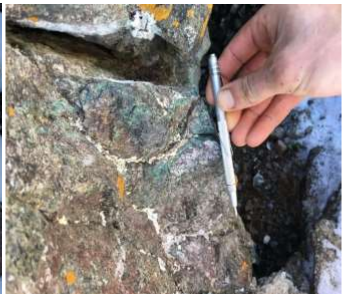
Copper-bearing calcite vein hosted by propylitically altered monzonite
