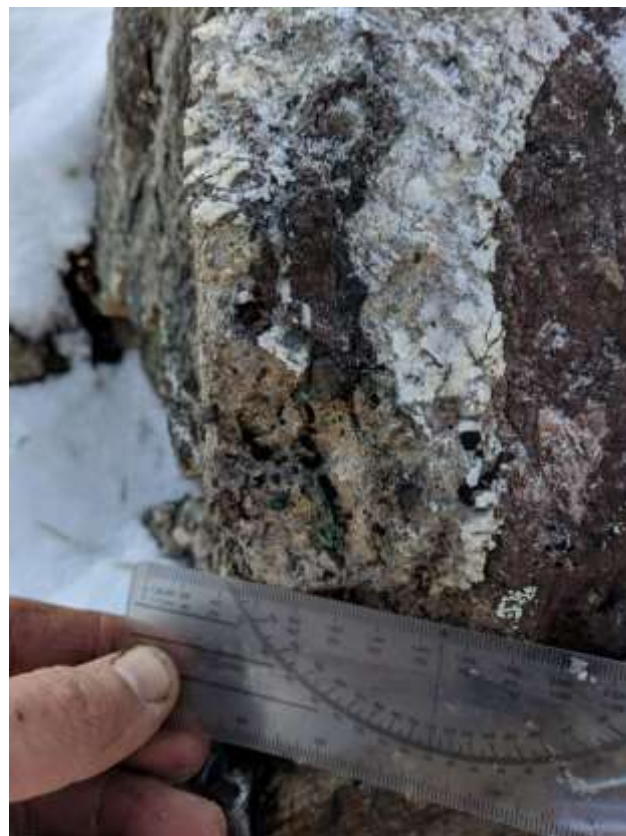
Calcite-chalcopyrite-malachite vein hosted by monzonite
