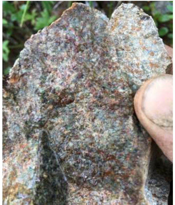
Iron carbonate and chlorite-epidote altered intrusive rock containing fine grained chalcopyrite, located approximately 600 m north of annular magnetic high.
