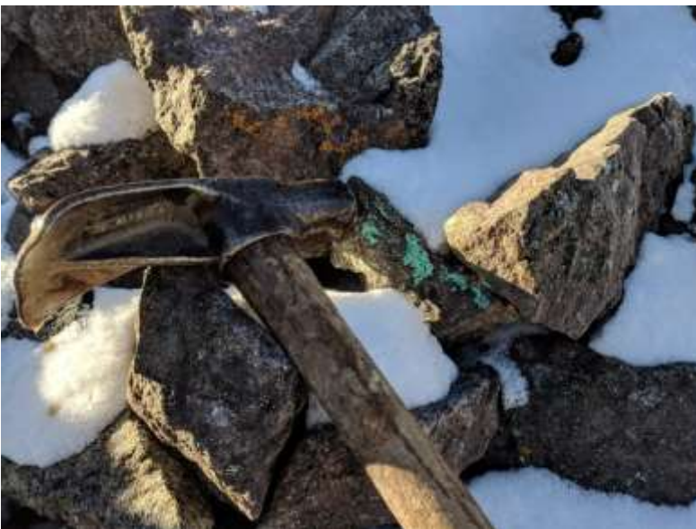
Chalcopyrite and malachite along fractures
