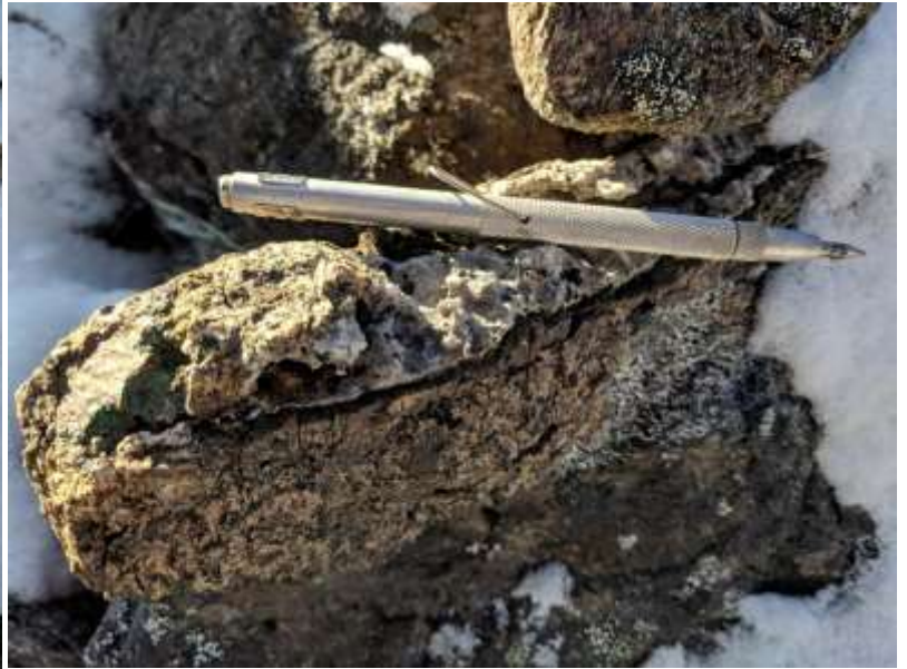
Detail of copper-bearing calcite veins hosted by monzonite
