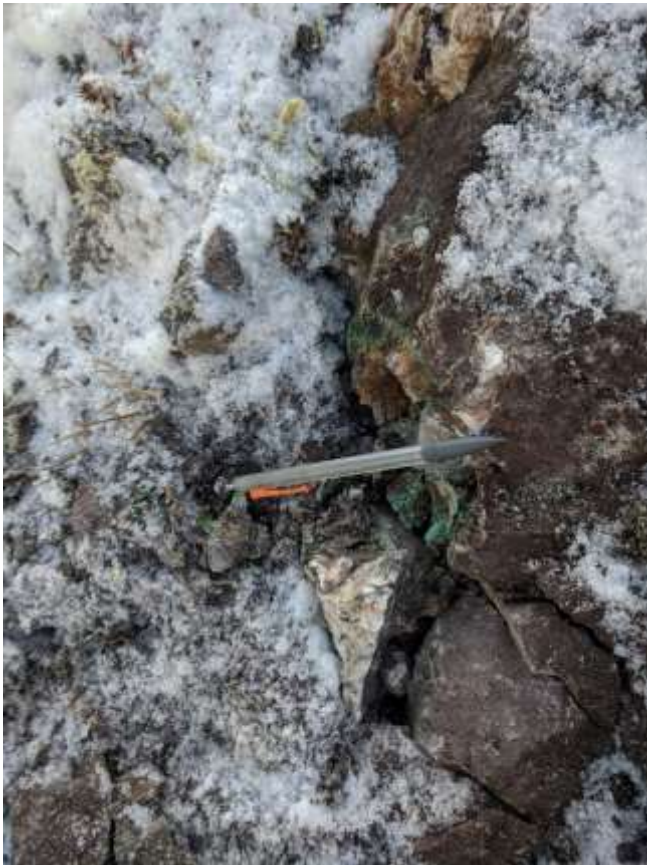
Copper-bearing calcite veining with malachite
